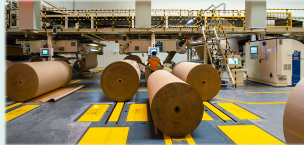
Automatic Paper Roll Mounting & Returning System (Paper feeding with a single button/ automatic paper returning)
